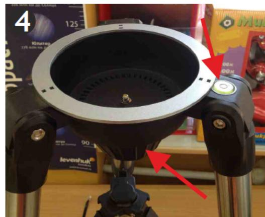
**EN** Tripod head without the mount. The clamping screw is in the center.
